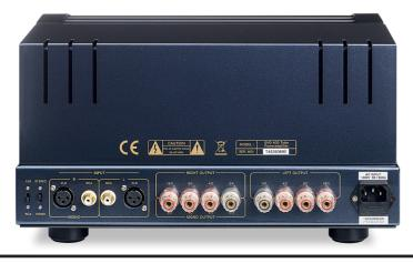
LEFT: The EVO 400 power amp has balanced (XLR) and single-ended (RCA) inputs, switched alongside. There are also three 4mm speaker outputs per channel fed from 16ohm, 8ohm and 4ohm transformer taps, respectively
