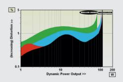
ABOVE: Dynamic power output versus distortion into 80hm (black trace), 40hm (red), 20hm (blue) and 10hm (green) speaker loads. Max. current is 9.0A
