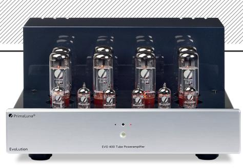
**ABOVE:** At 31kg, the EVO 400 power amp's bulk stems from the toroidal PSU transformer and two custom output transformers [all in screening can, behind]. Red LED on the fascia means the two pairs of EL34 pentodes (per channel) are configured in Ultralinear mode; green LED indicates triode mode
